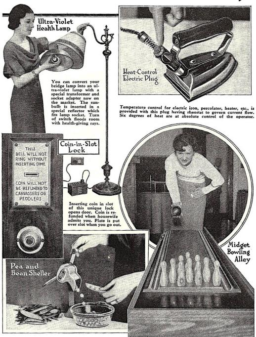
Labor of shelling peas is reduced to absolute minimum with this automatic sheller now on market. The peas are fed into the hopper with the left hand while the crank is turned with the right. The peas or beans roll out into the dish while the empty pods drop on the other side. Clamps to table as shown, and does a clean job of removing strings and separating peas and pods.
