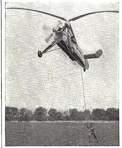
Pilot has perfect control of new Cierva 'gyro at all times, even when it is flying at speed slower than that of running man. Here a package is being picked up from dropped line.
