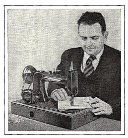
Attachment for sewing machine converts it into jig saw to cut out jig-saw puzzles. Handles wood up to 3/4" thickness.
